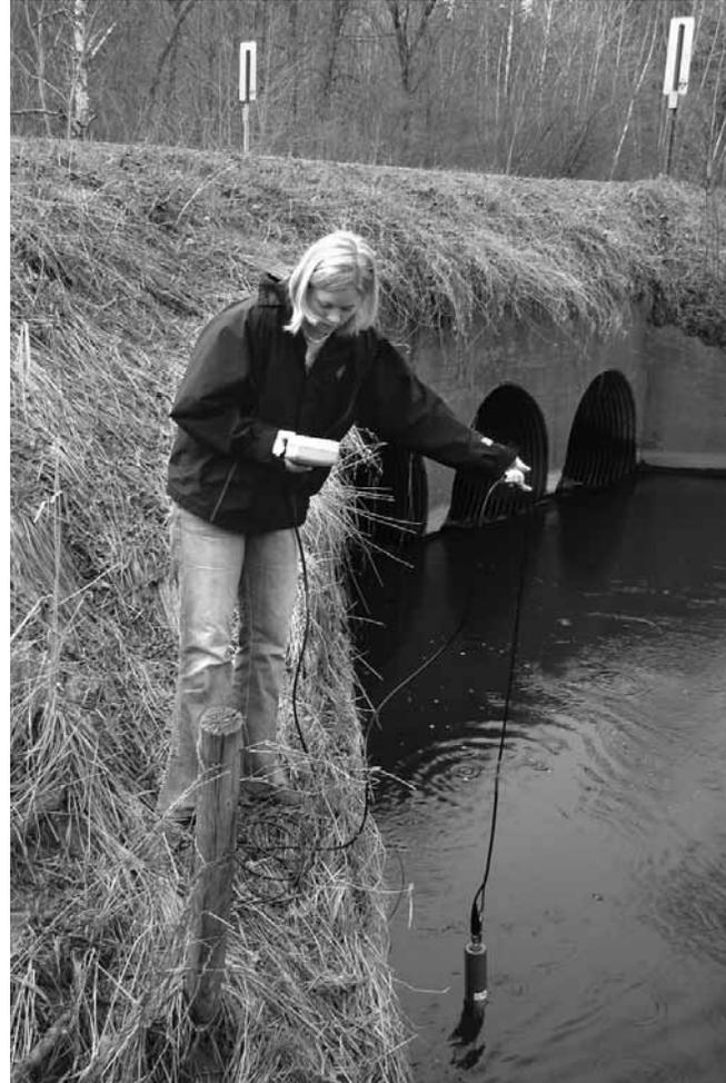
Chisago Soil and Water Conservation District Technician, Casey Ambers, uses a Sonde to measure and monitor levels of dissolved oxygen, conductivity, pH, temperature, and turbidity in the North Branch of the Sunrise River.
